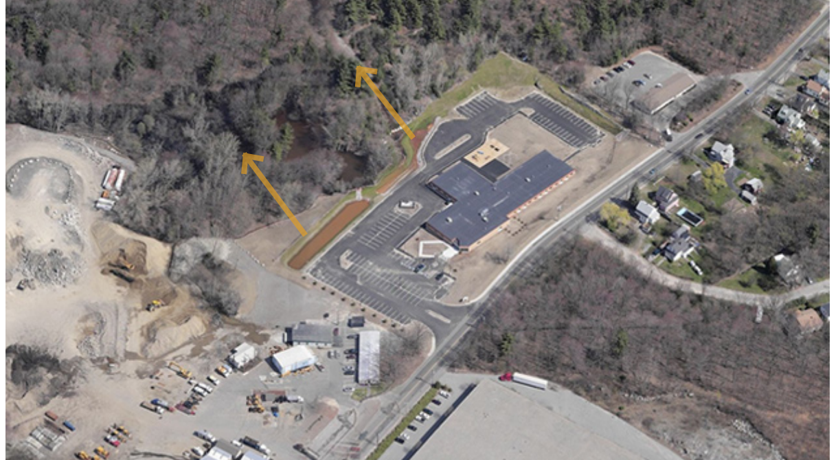
The detention basin adjacent to the school car park and the neighboring sand quarry does not have a sufficient buffer zone to adequately filter noxious effluent. Additional planting and a curb at the edge of the parking area will alleviate some of the ill effects of these adjacencies.
